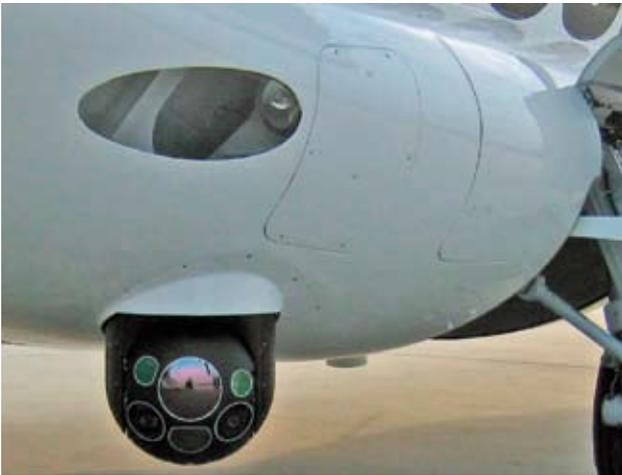
The turret of the electro-optical/infrared sensor
